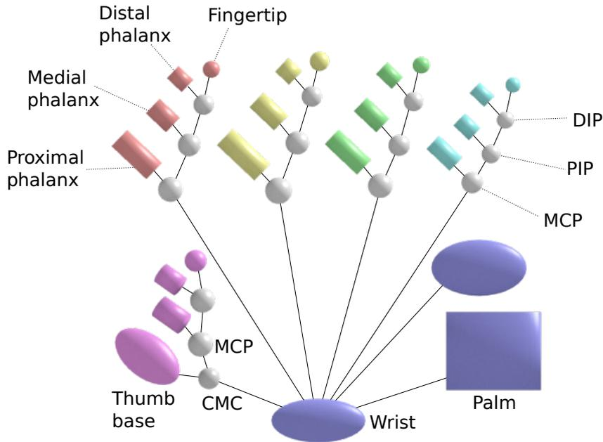
Figure 3.9: Full forward kinematics tree, with joints and shapes.
