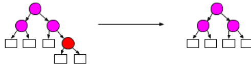
Figure 3.4: Example of prune in mutation. The red node is a revision point and will be erased from the tree.
