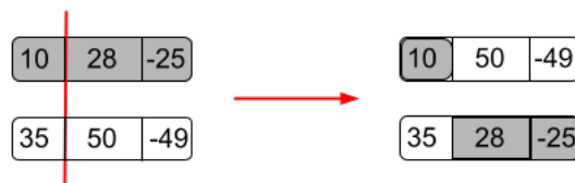
Figure 2.6: Example of crossover operator.
