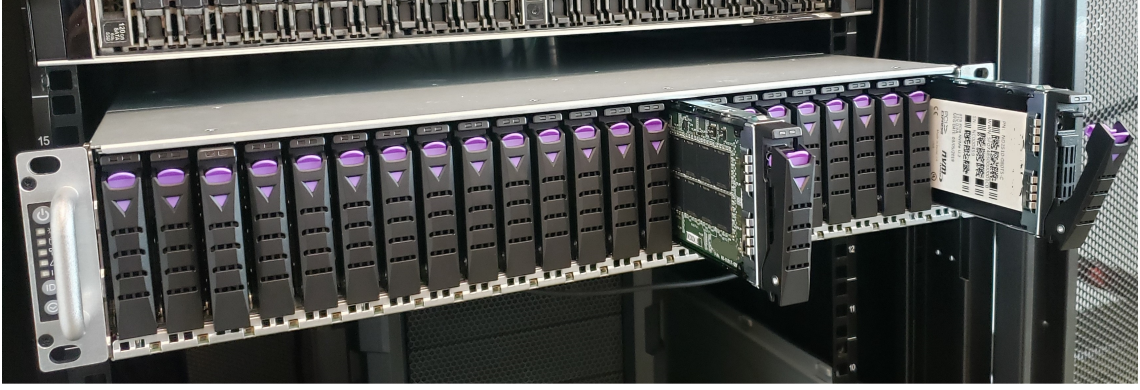
Figure 4.2: Experimental server blade with high capacity in-storage processing Newport CSDs. (Image from [1])
